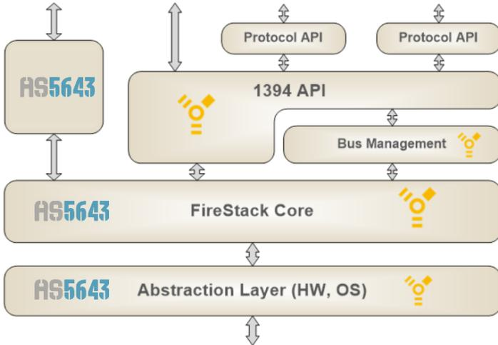
Conceptually, FireStack® addresses all these issues. It complies with IEEE1394 requirements as well as select higher protocol layers e.g. IIDC). And as the only product in the market it natively supports AS5643 features and functions. Due to the time critical aspects of that AS5643 protocol the AS5643 portion of FireStack® is only supported when running on top of an LLC with embedded AS5643 HW support (see FireLink® and FireTrac®).
