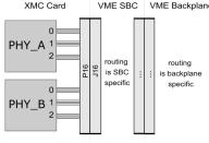
The following XMC-P16 pining has been assigned for 1394 bus signals:
