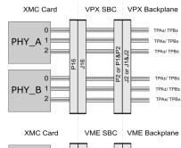
VME (VITA41.4) partial, availability of bus signals depends on the specific routing of signals from the P6 to P0 connector as well as backplane characteristics.
