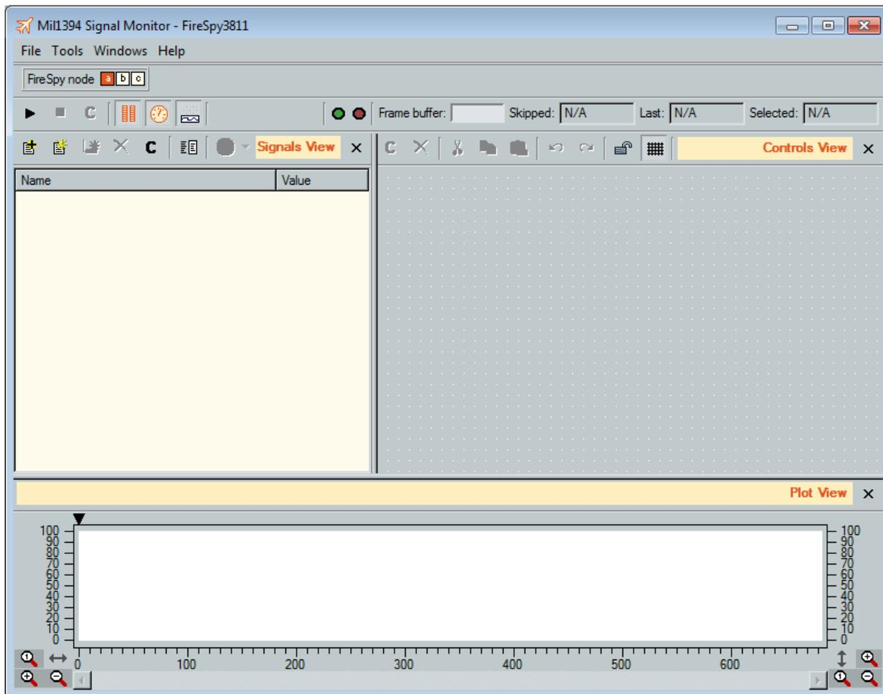
The easiest way to get started is to load the example file "Mil1394SigmonExample" that comes with the application. It already contains a set of signal definitions with some captured values also. After opening the file, the Mil1394 Signal Monitor will look like the following picture.
