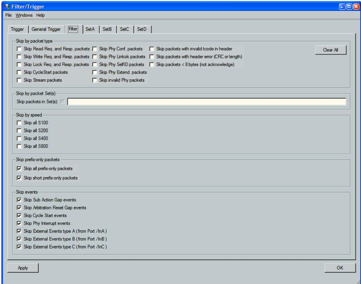
Using the **Skip by speed** box you can skip all packets of particular speed. When checking the Skip all S800 for instance, no S800 packets will be recorded.
