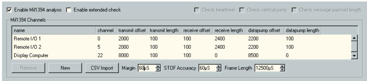
Note that you can also set the frame length, the frame length margin (i.e. how many microseconds the packet may arrive early or late) and the STOF packet accuracy. The latter is the amount of microseconds the next STOF packet may arrive early or late, in order not to be marked as invalid, relative to the prior one. These settings can also be defined in the XML file:
