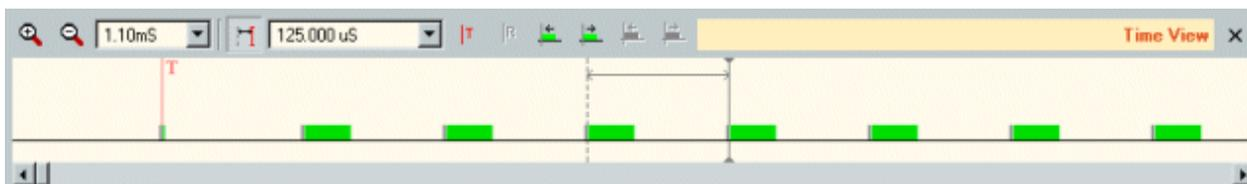
When in relative mode, clicking with the right mouse button will move both the reference and the cursor to the new location. This makes time measurements easier because you do not have to switch back to normal mode to move the reference.
