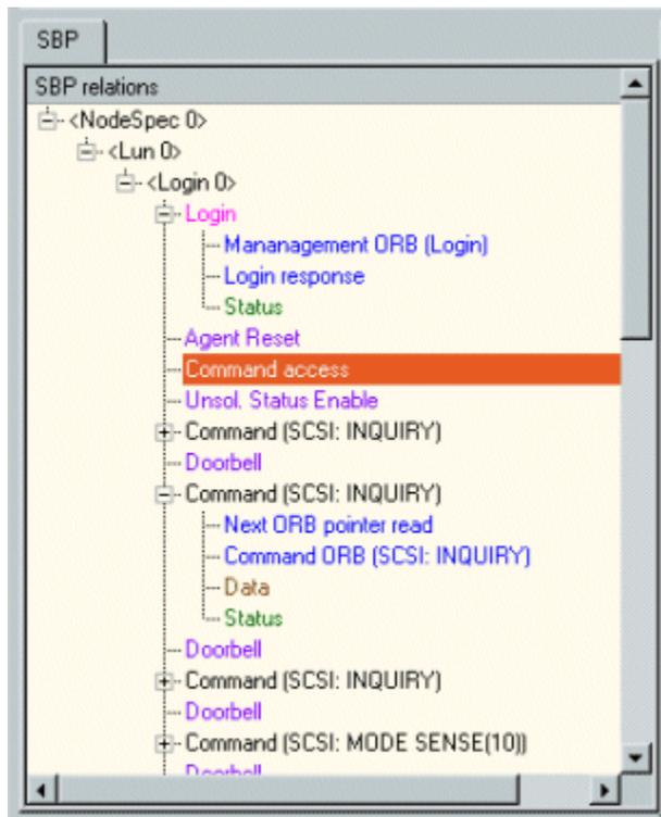
The hierarchy of the tree shows the nodes as root items, the units as child items of the nodes and the found results of the protocol analyzer as child items of the units. The terminology of the protocol determines how units and found results of the protocol analyzer are displayed in a tree, see also figure above. In a tree, the nodes are represented by their node specification ID. For more information about node specification ID, see [Protocol Settings](#).
