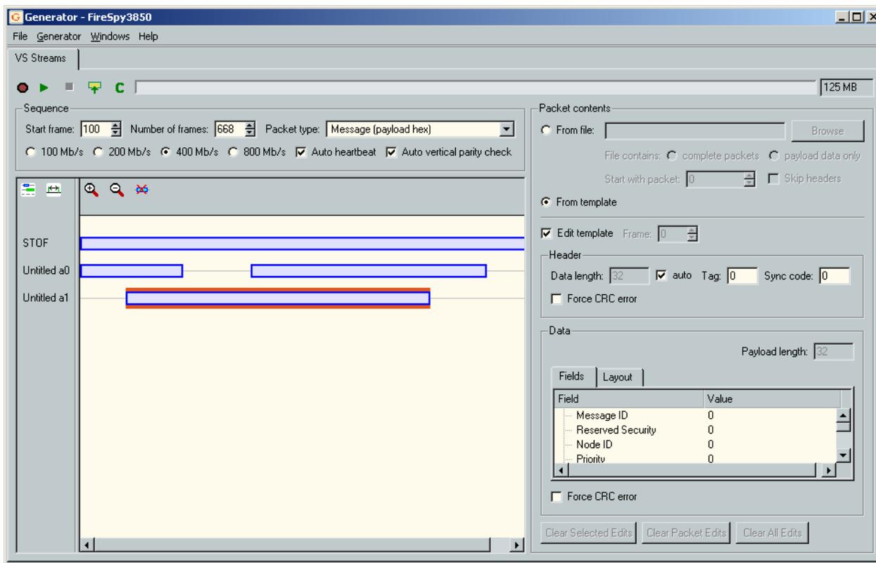
At the top of this window you can find the toolbar with buttons for starting, uploading and stopping the Generator. Before starting the Generator, you first have to upload the generator data to the Analyzer. This data can be specified in the "Mil1394 Streams" generator page, where you can define isochronous sequences. Sequences are indicated by blue rectangles on the time line of a slot. This can be seen in the picture above.
