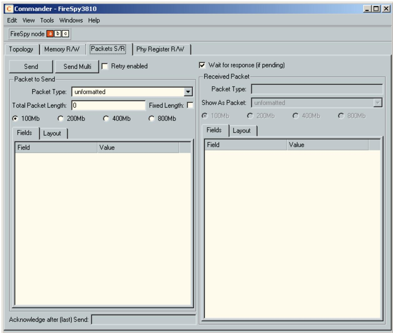
The send packet will be sent when you press the 'Send' button. If an acknowledge has been received for the packet, it will be displayed left at the bottom of the page. If retry is enabled, the packet will be retried up to 15 times if needed. The packet is retried if the target node did not respond with an acknowledge, or if it is acknowledged with an `ack_busy` or `ack_tardy` code.
