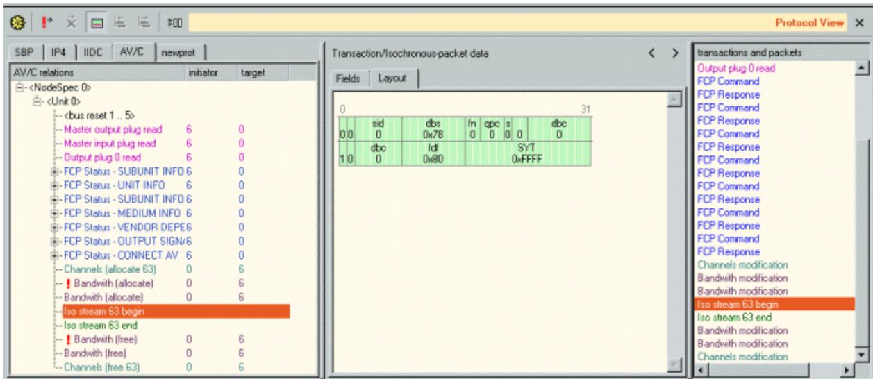
Protocol AV/C shows only the fields and their values of the highlighted transaction in the 'transactions and packets' pane and offers navigation buttons to walk through the corresponding transactions of the highlighted item.
