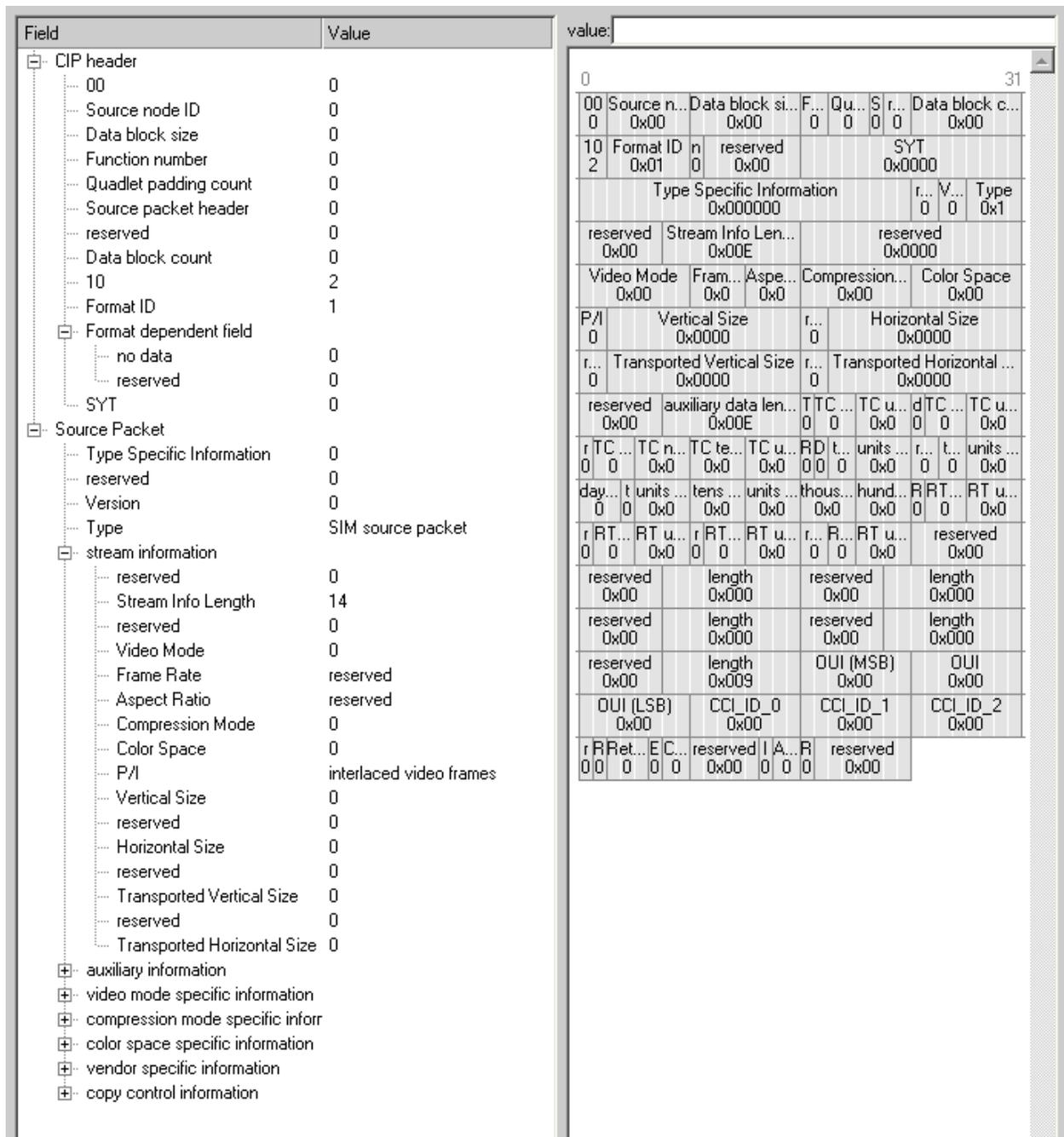
Using BT601 protocol audio and video data can be transferred uncompressed or compressed. Depend on the data format packet has different size, but header remains the same. Figure below shows BT.601 video
