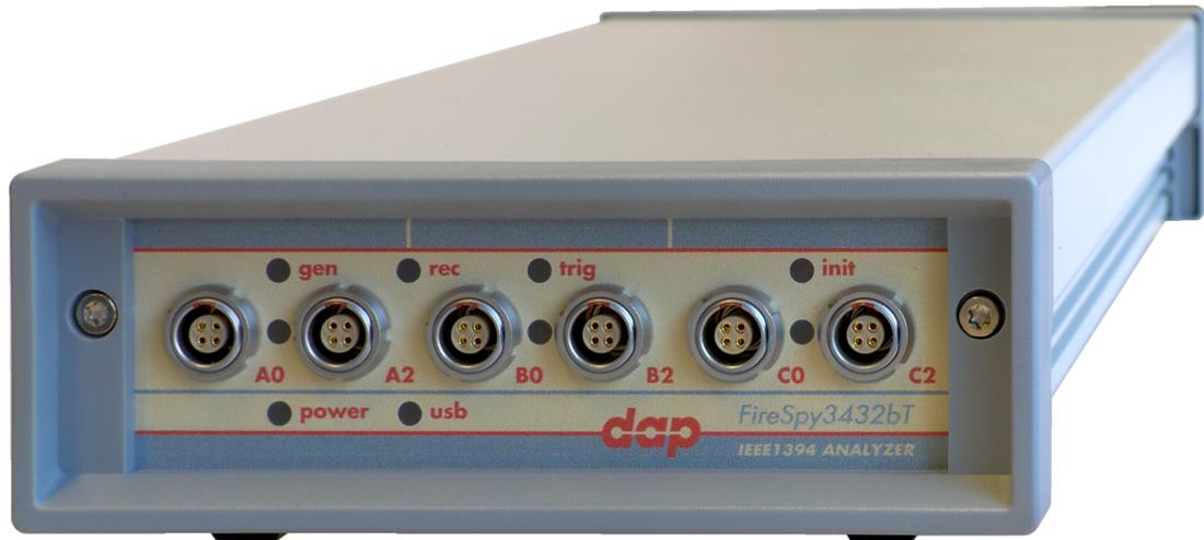
The FireSpy3x32bT has three 1394 nodes connected to three synchronized analysis engines. They are controlled by a dual core ARM processor running at 667MHz. Each node is connected to three 1394 ports. Two ports of each node are connected to a separate LEMO connector which was chosen over standard 1394 connectors for improved ruggedness.
