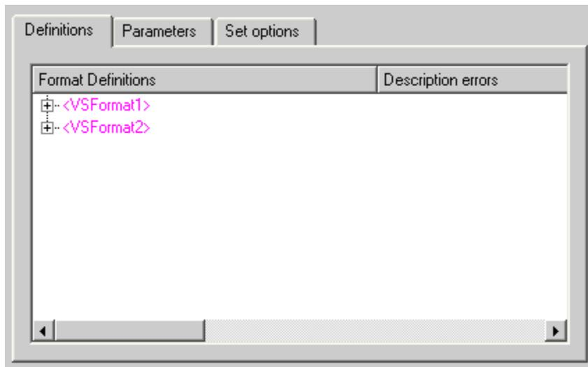
The upper tree format definitions (color magenta) are definitions available for the Analyzer. The 'command' and 'data' format definitions must be present to implement a correct command set. The format definition 'status' is only needed when the status format differs from the standard SBP2 status format. The other definitions (color blue) are macro definitions, used by the upper tree definitions.
