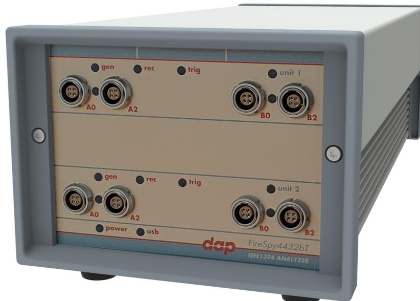
The FireSpy4x32bT has four 1394 nodes connected to four synchronized analysis engines. They are controlled by two dual core ARM processors running at 667MHz. Each node is connected to two 1394 ports. Both ports of each node are connected to a separate LEMO connector which was chosen over standard 1394 connectors for improved ruggedness.
