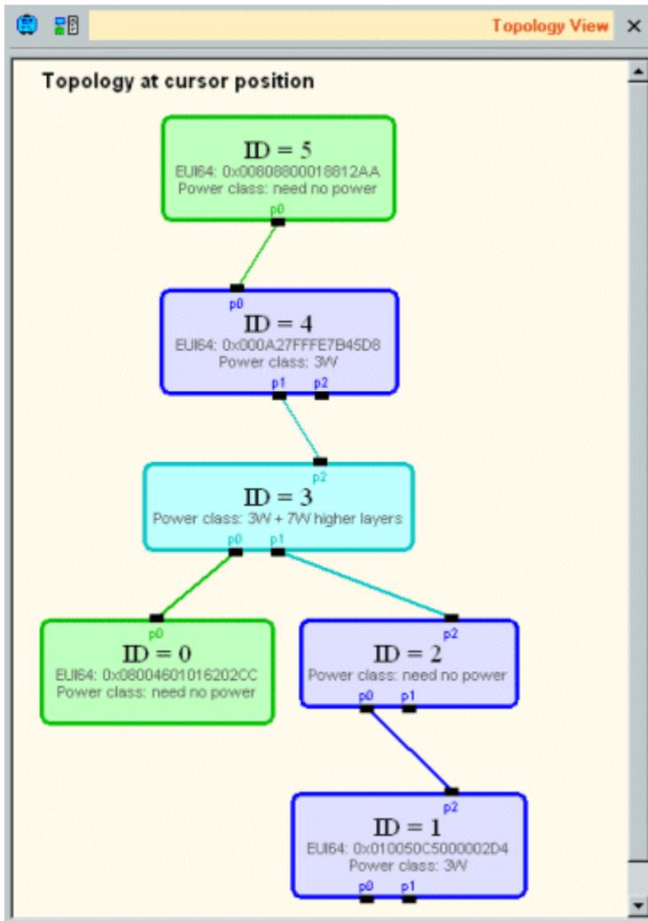
Using the 'Bus and node information' button (right button in Topology Toolbar) you can display additional bus and node information. In the example below this option is switched on. The extra node information corresponds to node 5, the selected node.
