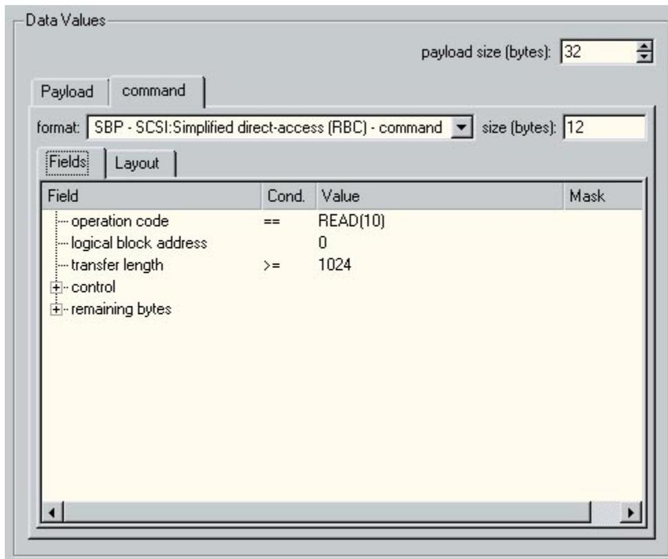
Depending on the license keys that are installed, you can select all kinds of formats and optionally sub formats where needed. There are formats for the SBP protocol, IIDC protocol, IP4 protocol and AV/C protocol. You can also select the format 'unformatted' to be able to set any kind of condition on any bits. Now we will describe the different parts of the Data Values box:
