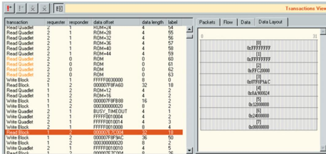
For Lock transactions the tree data values (argument, data and old data ) are now displayed underneath each other. The example below shows the same Lock transaction as the lock transaction above the previous example.
