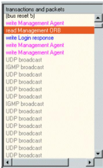
The 'transactions and packets' pane may list transactions and packets of multiple protocols. If this is the case all transactions and packets of the protocol of the highlighted item in the 'relations' pane are displayed in their normal text color and all transactions and packets of the other protocols are displayed with a gray text color, see also figure above.
