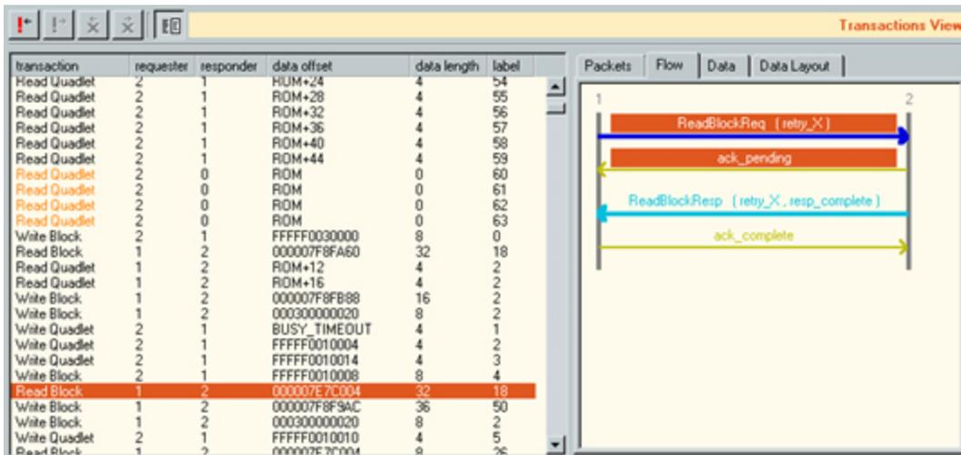
As you can see above, the retry-code, response-code and acknowledge codes are also displayed in the flow graph, so that you easily can see how the transaction is build up.
