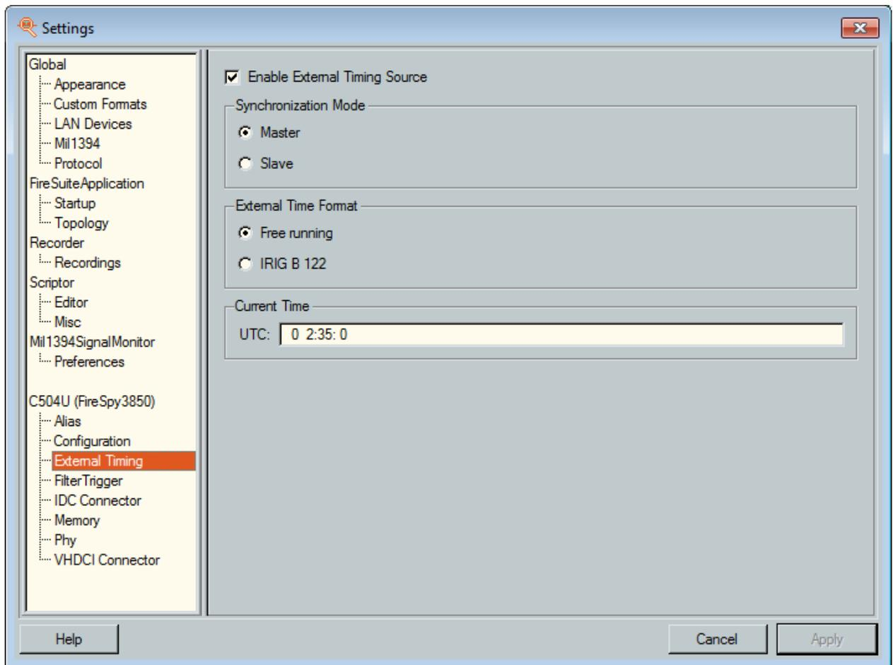
The FireSpy385X is capable of synchronization between multiple analyzers by setting one as a time master and the others as time slave. Time on the master can be configured either using an internal clock running in free running mode or using an IRIG timing source (in combination with a DapTechnology IRIG Demodulator) to synchronize the internal clock. Currently the Recorder is the only module capable of using the external timing.
