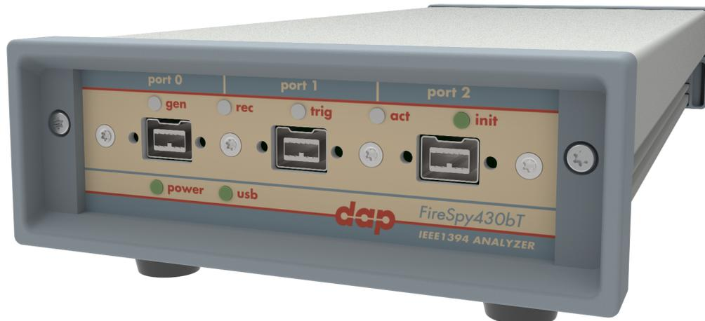
The FireSpyx30xx has one 1394 node connected to one 1394 analysis engine. It is controlled by two dual core ARM processors running at 667MHz. Its 1394 node is connected to three 1394 ports. All ports are connected to a separate IEEE-1394 connector with screw mount holes which was chosen over standard 1394 connectors for improved ruggedness.
