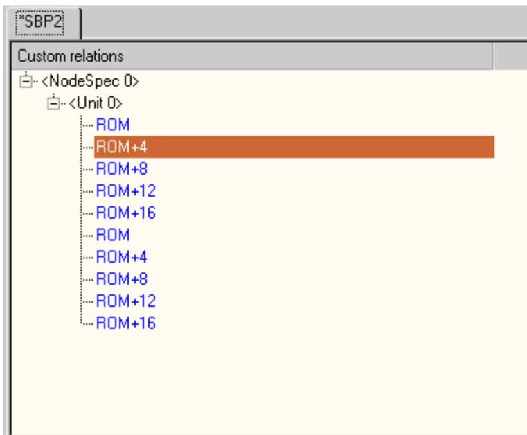
For each found or manually specified NodeSpec there will be a root item in the tree (NodeSpec 0 above). For information about NodeSpec's, see 'Custom-made Protocol Settings' below. For each found or manually specified Unit, there will be a Unit item inside the corresponding NodeSpec (Unit 0 in NodeSpec 0 above).
