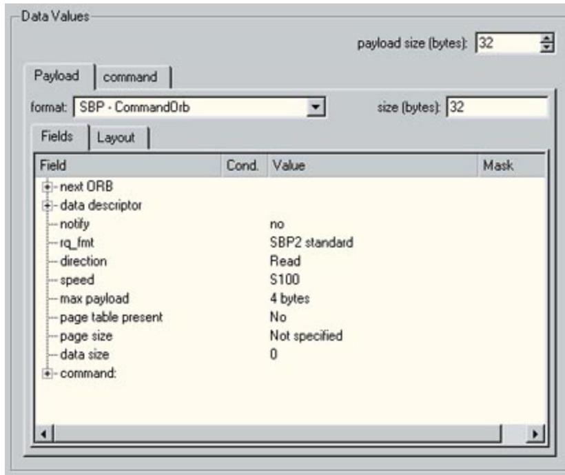
The fields in the table show the fields for the payload of this packet format. You can put conditions on these values just as could be done with the header fields. If the format of a packet depends on the value of one of its fields, the format will automatically be adjusted if you change the value of that field.
