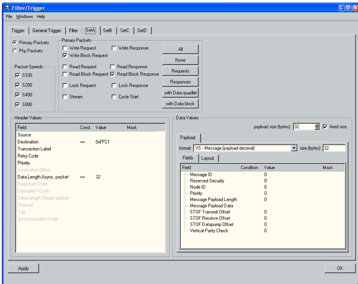
In the **Header Values** box, you can specify conditions for header fields. Only packets for which the specified conditions are met will fit the set. The table in this box shows all possible fields that can be present in a 1394 packet header. Only those fields that are present in the selected packet types will be enabled. You can only specify conditions for those enabled fields. If more packet types are selected, only those fields will be enabled that are present in all the selected types.
