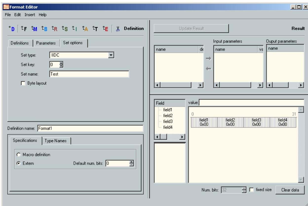
A set should always be of one of the known "Set Types". This enables automatic loading by the Analyzer application. Furthermore, the field "Set name" should not be set to "general" as this name is used by all
