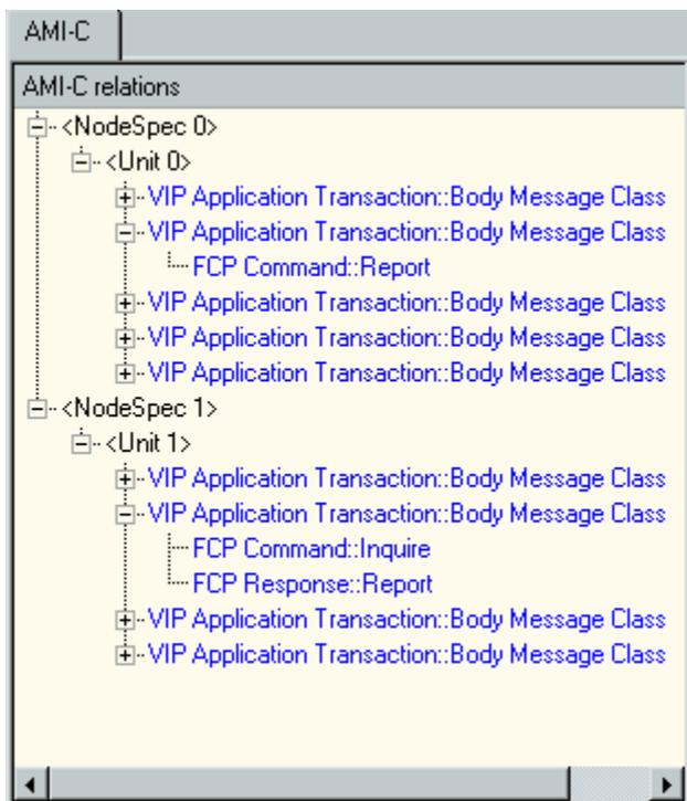
For each found or manually specified NodeSpec there will be a root item in the tree (NodeSpec 0 above). For information about NodeSpec's, see 'IP4-Protocol Settings' below. For each found or manually specified Unit, there will be a Unit item inside the corresponding NodeSpec (Unit 0 in NodeSpec 0 above).
