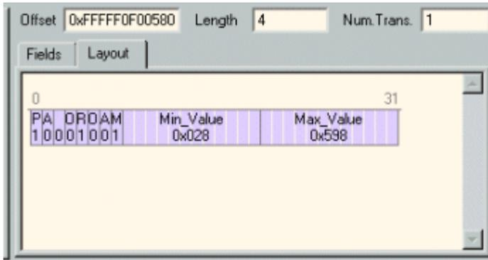
If a Bandwidth allocation/de-allocation or Channel allocation/de-allocation or Plug register transaction is selected, the 'Layout' page displays the data corresponding to a lock transaction. For lock transactions, the 'Argument' layout is drawn on the top, the 'Data' layout in the middle, and the 'Old data' layout at the bottom. See below for an example of the layout for a bandwidth allocation lock transaction.
