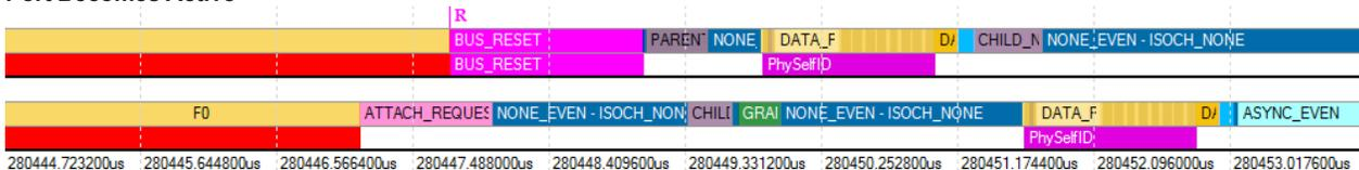
After the port detects making it active will not result in a loop, it sends an ATTACH\_REQUEST which is responded with a BUS\_RESET control. (See Chapter 14.7.9 and 14.7.10 of the specification).
