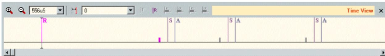
In this example a Bus Reset occurred, followed by two Phy-SelfID packets. After the second SelfID packet there is for some time no packet, resulting in the Subaction Gap and Arbitration-Reset Gap events. Then a cycle-start packet is transmitted and again a while nothing, resulting in the Subaction Gap and Arbitration-Reset Gap again, etc.
