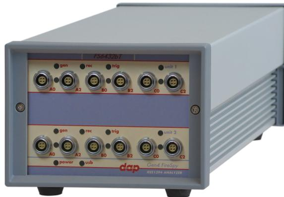
The FireSpy6x32bT has six 1394 nodes connected to six synchronized analysis engines. They are controlled by two dual core ARM processors running at 667MHz. Each node is connected to two 1394 ports. Both ports of each node are connected to a separate LEMO connector which was chosen over standard 1394 connectors for improved ruggedness.
