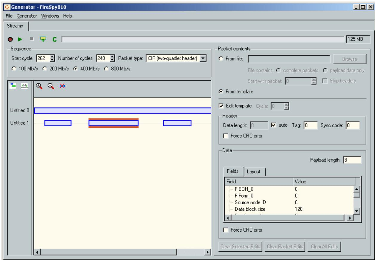
At the top of this window you can find the toolbar with buttons for starting, uploading and stopping the Generator. Before starting the Generator, you first have to upload the generator data to the Analyzer. This data can be specified in the "Streams" generator page, where you can define isochronous sequences.
