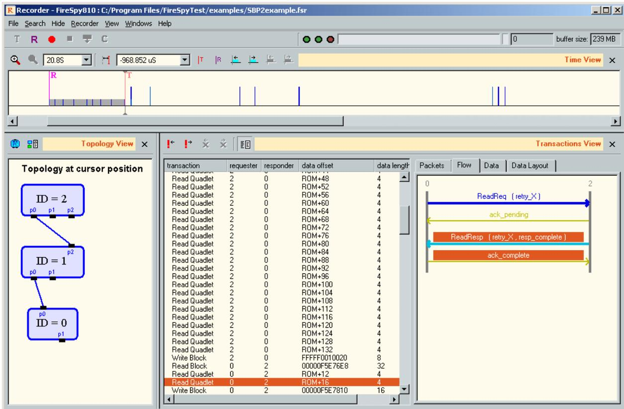
You can use the 'Recorder' menu or toolbar buttons to record packets into internal memory of the Analyzer, and download them to the host. The recorded data can be viewed in the same way an opened file can be viewed. The recorded data can also be saved to disk as a Analyzer recorder file using the 'Save As' command in the 'File' menu. In this 'File' menu there is also an 'Export Packets' command, which can be
