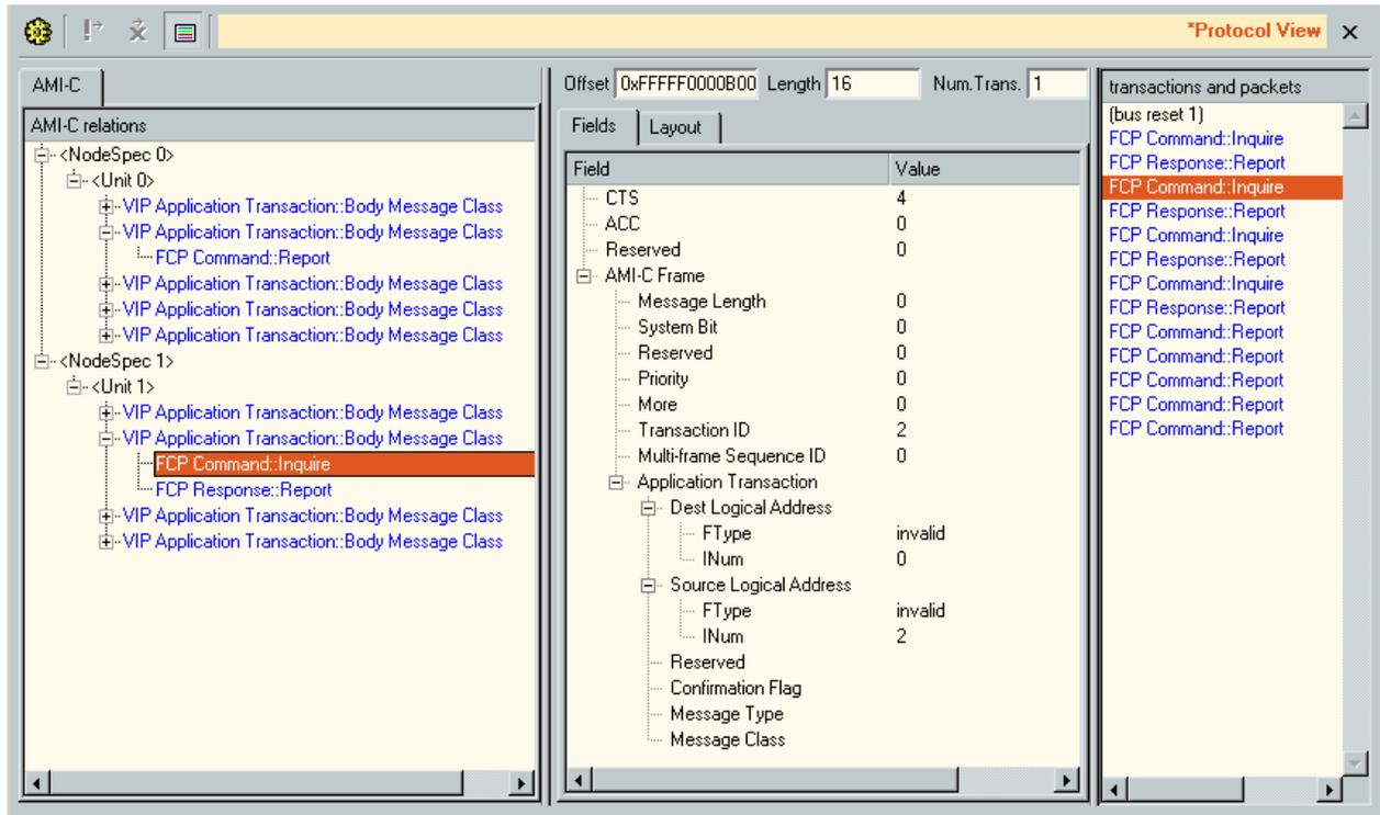
It displays the result in three different parts. At the right (transactions and packets), all found packets and transactions are displayed in the order they were detected on the bus. The left part (relations) shows the relation between these items. The transactions and packets belonging together (e.g. all transactions that form a single FCP command) are grouped into tree items and these items are displayed hierarchically in the 'relations' pane. In this tree you will find for instance:
