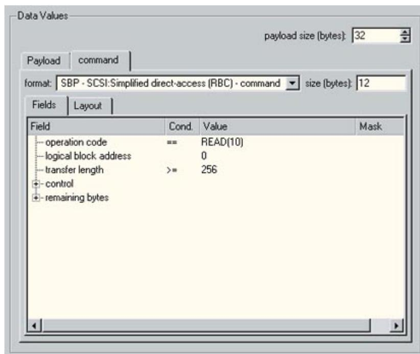
Depending on the license keys that are installed, you can select all kind of formats and optionally sub-formats where needed. There are formats for the SBP protocol, IIDC protocol, IP4 protocol and AV/C protocol. You also can select the format 'unformatted' to be able to set any kind of condition on any bits. Now we will describe the different parts of the Data Values box:
