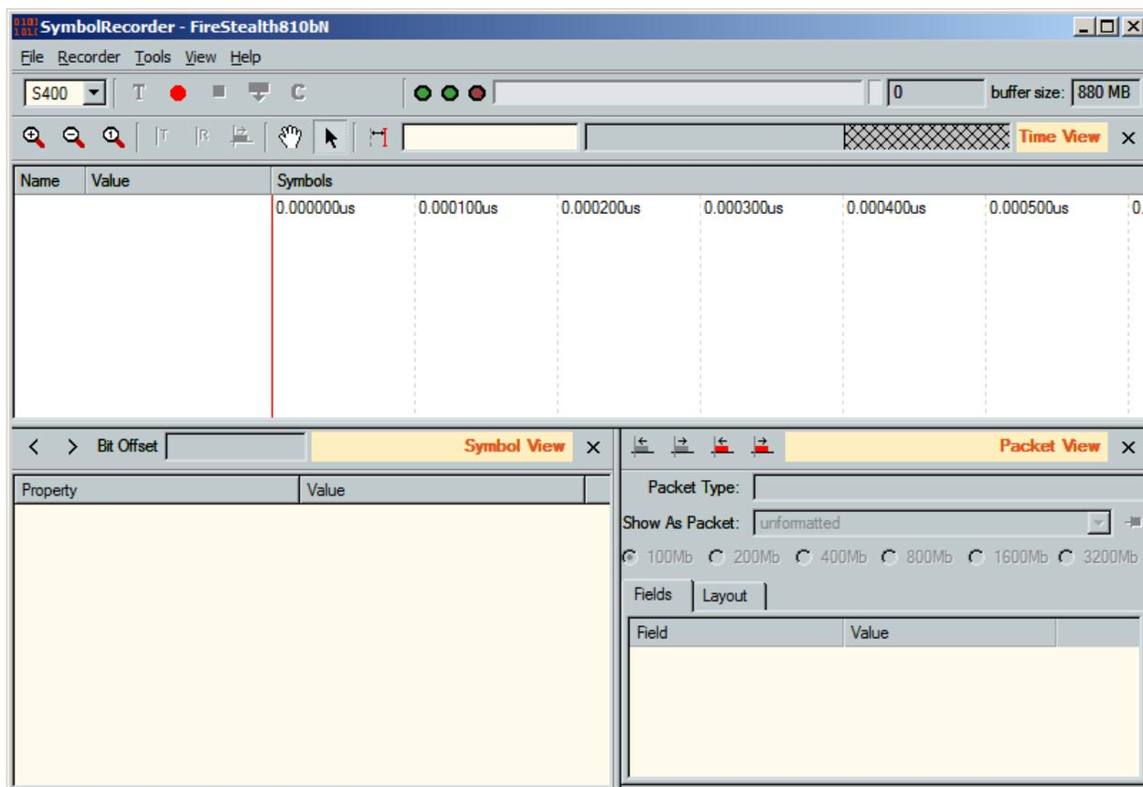
The window is filled with different kinds of views for the recorded data. You can switch them on and off. The Time View is always displayed (if enabled) at the top. The remaining views share the area between them. You can enable and disable the different kinds of views using the 'View' menu. In the picture above, the Time View, Symbol View and the Packet View are visible.
