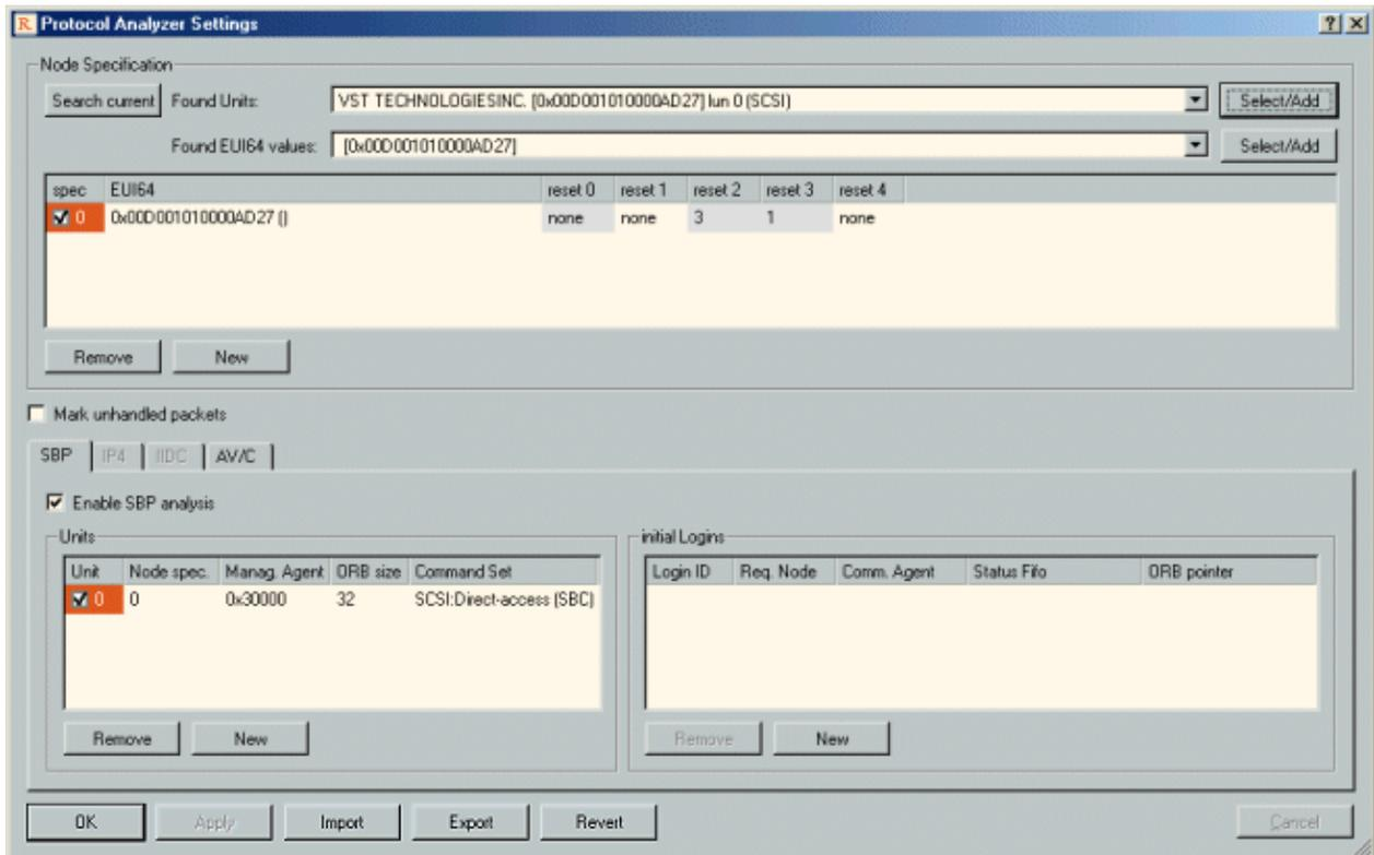
Mostly the protocol analyzer will need information about the Units inside the nodes that comply to the protocol. For example the SBP protocol will need to know which nodes contain SBP Units and for these Units it needs to know the 'Management Agent', 'ORB size' and supported 'Command Set'. All this information can be found in the Configuration ROM of the node. The analyzer will search for Configuration-ROM reads to find out this information automatically.
