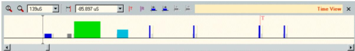
The cursor is a vertical line with little triangles on the top and bottom, as shown above (left to the first packet).
