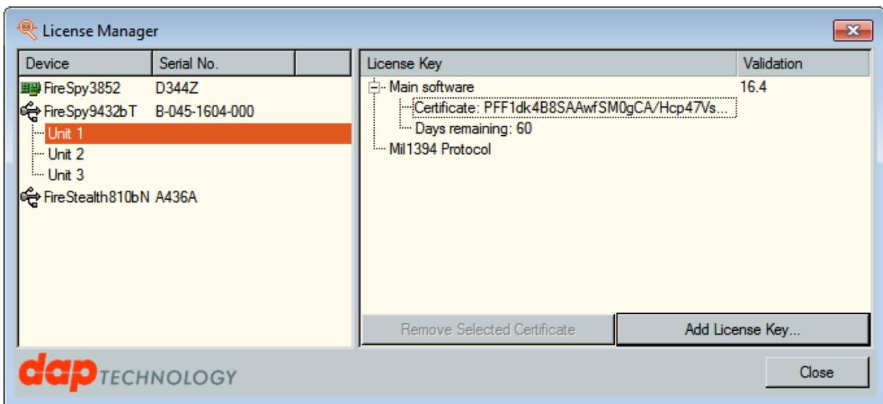
You can add keys with the 'Add License Key...' button or remove them by selecting a key and clicking the 'Remove Selected Key' button. You will need to restart the application to activate the new keys, except in the startup dialog; licenses added there can be immediately used.
