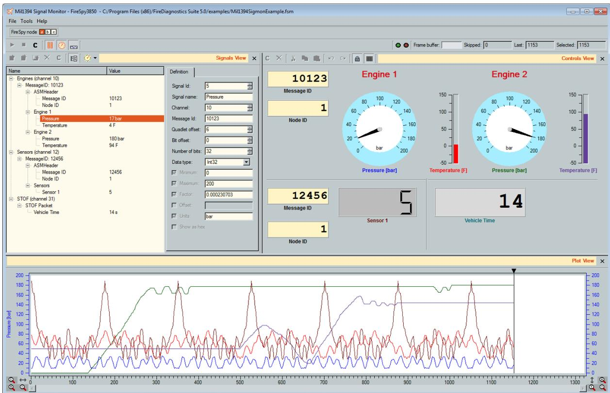
Using the cursor line in the plot view at the bottom you can navigate through all the frames and show the signal values captured in a specific frame number.
