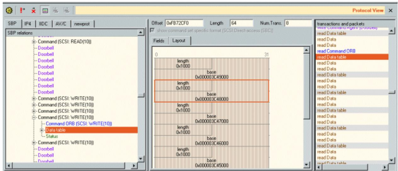
In the figure above, the red frame indicates the highlighted transaction or packet in the 'transactions and packets' pane. The Fields tab page of the 'detail' pane is shown in the figure below.
