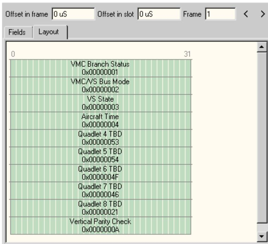
Like the 'Fields' tab page it shows the fields and their values of the highlighted Mil1394 packet. But now the fields and their values are displayed graphically inside a data block, which represents the highlighted Mil1394 packet.
