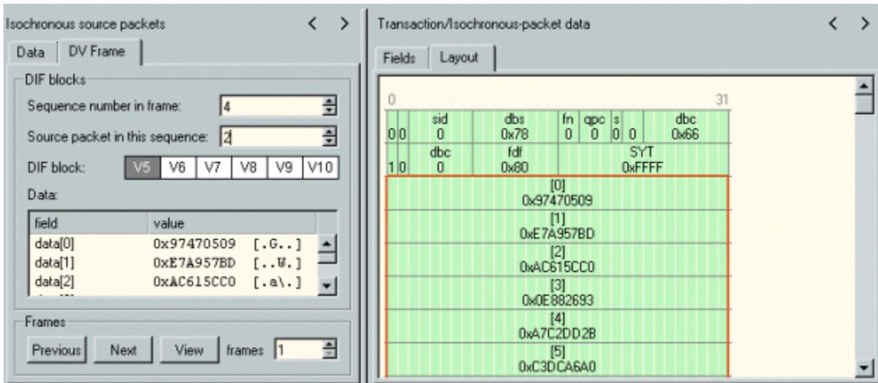
The DV-Frame tab can be used to walk through the logical data inside an isochronous video-frame packet. Each source packet consists of a series of DIF blocks. Using the edit control with spin box labeled 'Source packet in this sequence' all parts of the DIF block can be displayed. Clicking on a DIF block will display the content of that DIF block in the 'Data' table. Using the edit control with spin box labeled 'Sequence number in frame' all sequences in a video frame can be selected.
