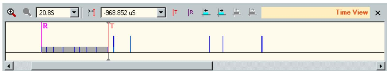
At the top of the view you see a toolbar with some buttons and controls like zoom in and zoom out buttons, the cursor time indicator and buttons to quickly find other packets of the same type as the current selected one or packets with errors. Below the toolbar is the time line. It is a horizontal black line with the packets and events drawn on top of it.
