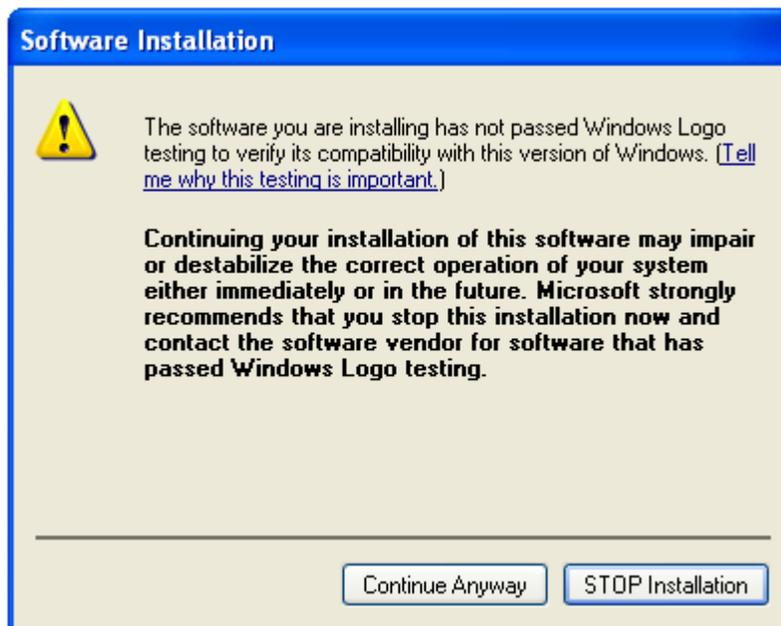
During the installation of the Drivers, the following message may be displayed, saying the driver certificate has expired. As with the Windows Logo testing, the FireSpy driver signing is not supported for older Windows versions. Click "Yes" to continue installing the driver. This message may appear once or more during installation, depending on the number of FireSpy devices connected to the machine.
