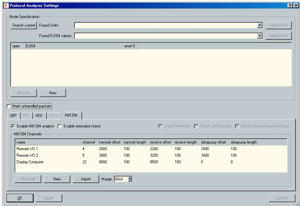
The information of the nodes, which support the Mil1394 Protocol, is to be added in the table 'Mil1394 Channels' of the Mil1394 tab page. Click on the Mil1394 tab to show the Mil1394 tab page on top.
