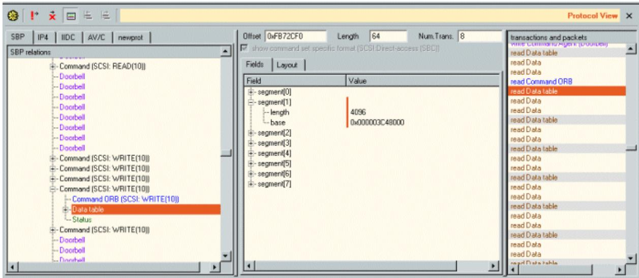
The red bar indicates the highlighted transaction in the 'transactions and packets' pane, which is in this case the second corresponding transaction of the highlighted item in the 'relations' pane.
