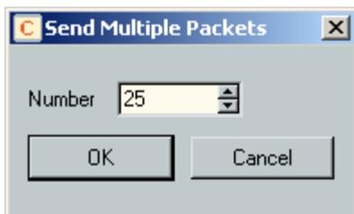
If the user enters a number equal to, or bigger than 1, and presses 'OK', the application proceeds to send the packet the selected number of times in rapid succession. If the packet(s) sent result in response packet(s), only the last one received will be displayed in the Packet S/R window.
