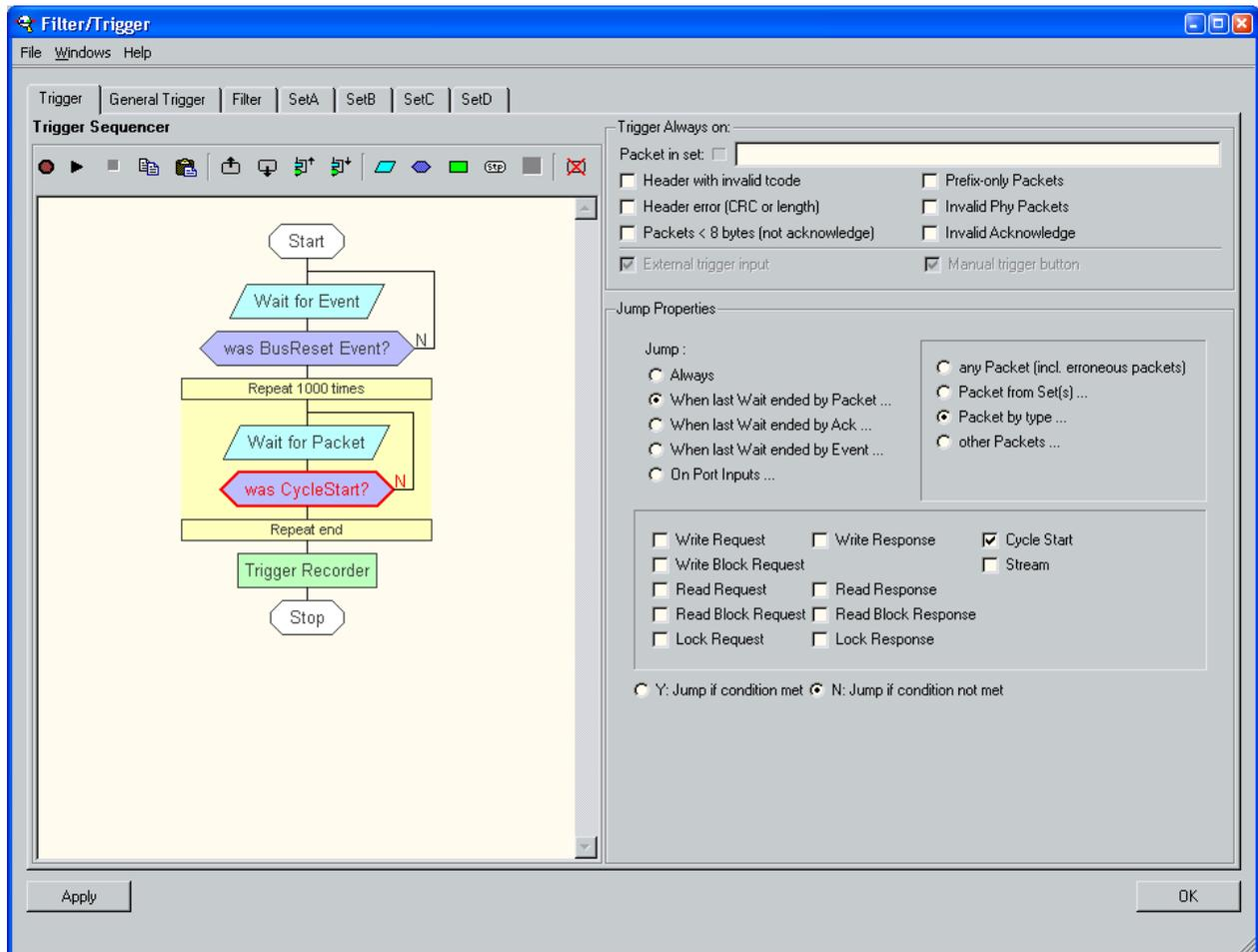
The most important part for the trigger settings is the **Trigger Sequencer**, see left pane in example above. Here you can graphically define a trigger program by adding items to the flow and change their properties. By executing the program you can generate a Recorder trigger when a particular sequence of packets or events has been detected.
