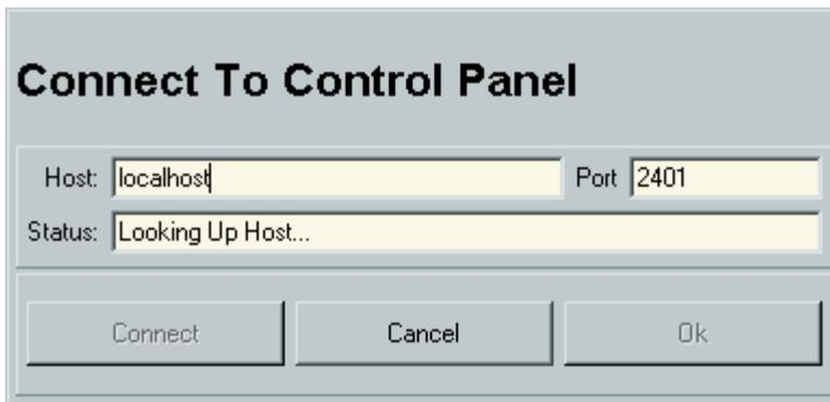
This dialog has two input fields, the host it must try to connect to and the port number. Because the communication between the Analyzer application and the client uses TCP/IP you need an IP address or a computername and a port number. The Analyzer application only accepts connection when the same icon is selected.
