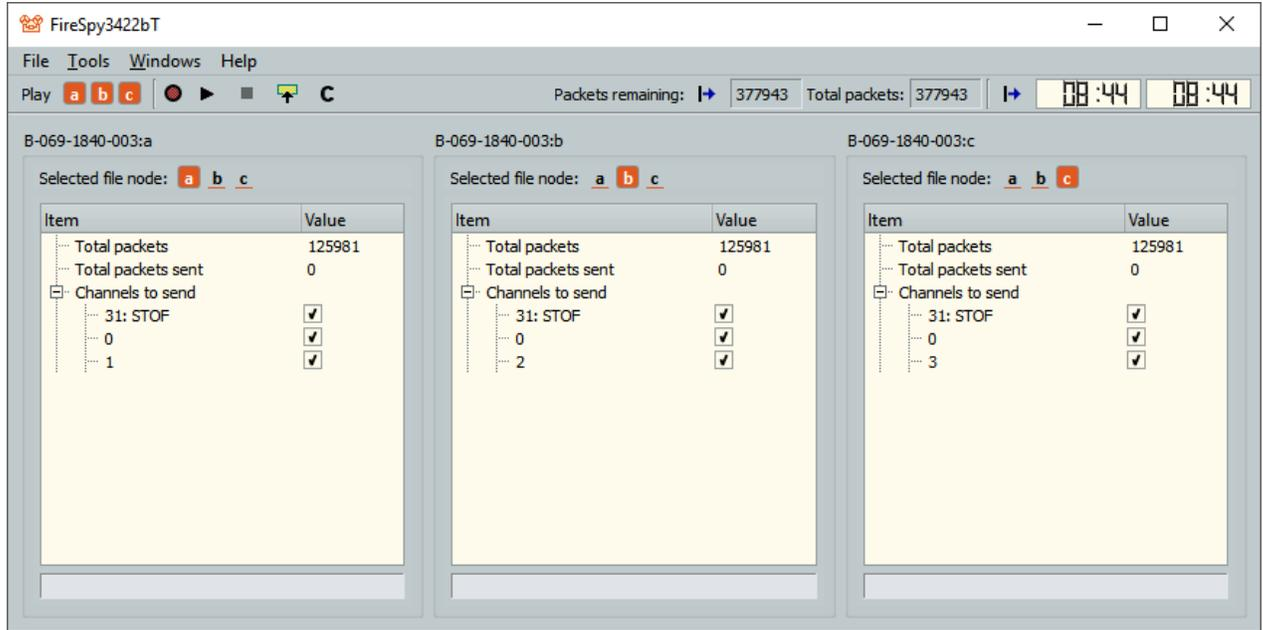
To play the selected Regeneration file, simply click the Play button in the toolbar at the top. This will upload the Regeneration data to the FireSpy, and play the stream packets on the FireSpy nodes. Use the Upload button will only upload the data to the FireSpy, without starting the Player.
