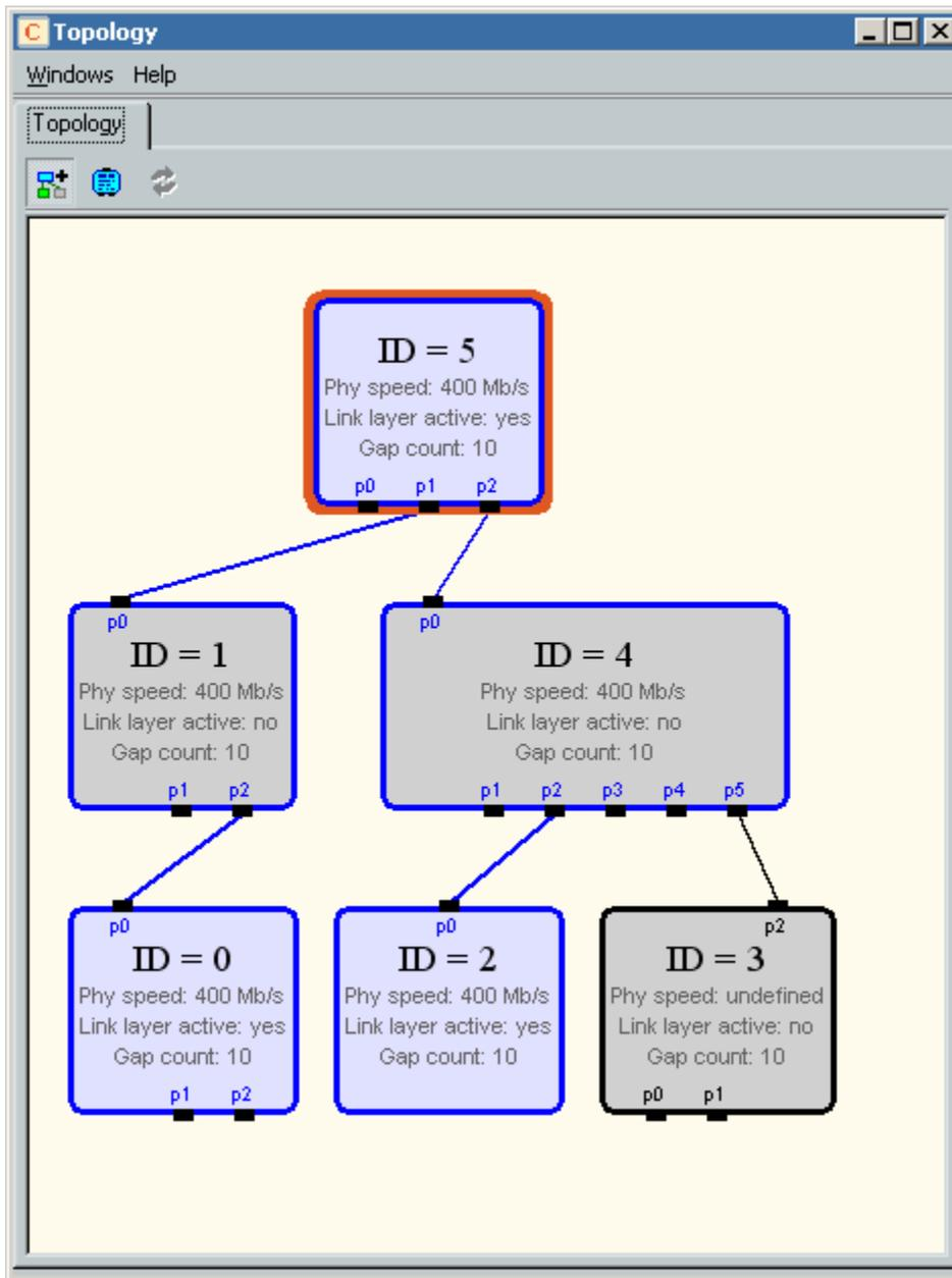
Whenever configuration of the FireStealth is done after configuration of the 1394b bus, the FireStealth will have missed the IEEE 1394b bus configuration and will not be able to gather the bus topology information.
