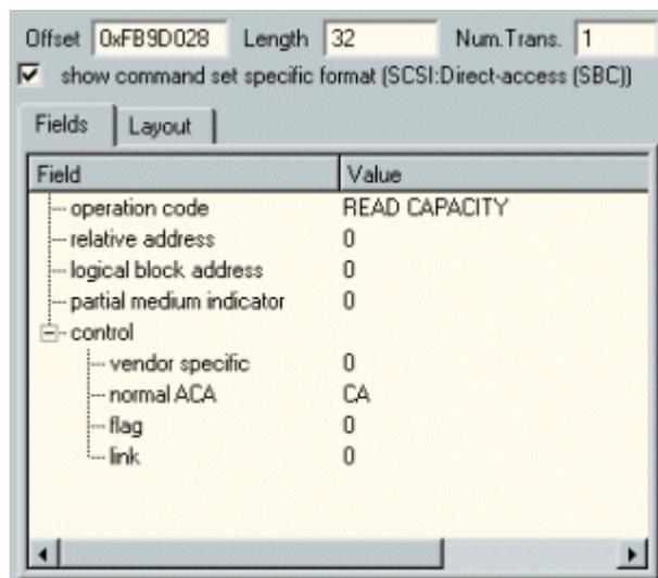
When the 'show command-set-specific format' option is selected, only the command-set-specific part is displayed. In the example above, the same item is selected, but now only the 'command block' is shown. It is formatted according to the format set defined in the SBP-Protocol Settings (see below). The used command set is also shown after the check box. In the example above it is the SCSI-Direct-access (SBC) command set.
