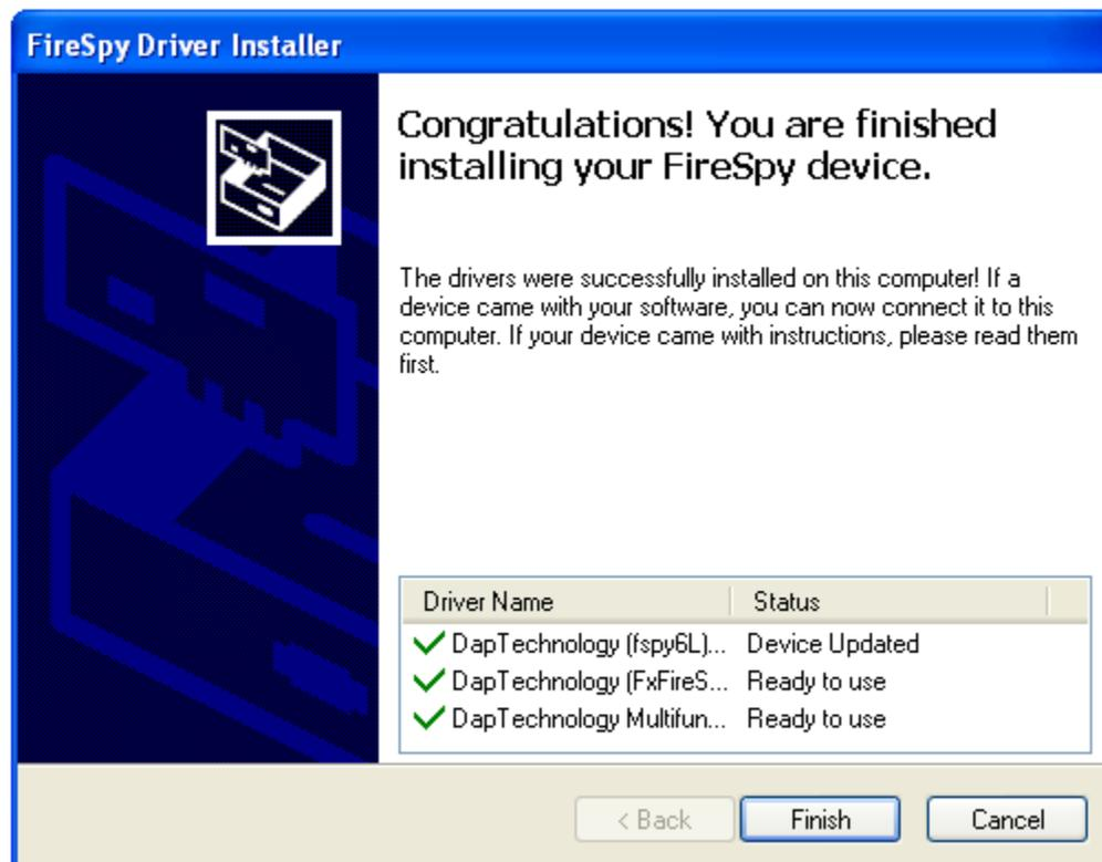
Any devices that were connected to the machine during the installation should work now. If there were any unplugged devices, please connect them to the machine now. The Windows Driver Wizard mentioned earlier should appear now. If it doesn't please reboot the machine. In the Driver Wizard, select the bottom option "No, not this time" to search for the already installed drivers, and click "Next" to continue.
